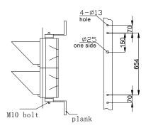
2. Installing traffic lights the visors JD200 signal sun on
